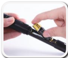
2. Insert a AA battery
