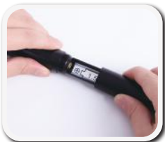
1. Unscrew the battery case
