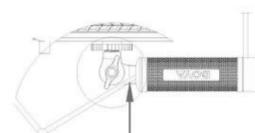
2) Loosen the knob and adjust to desired angle
