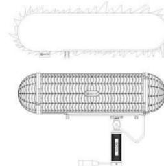
2) Straighten the fur windshield, then tighten and lock the drawstring
