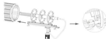
2) Tighten the front and rear knobs
