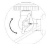
3) Tighten the knob after adjustment
